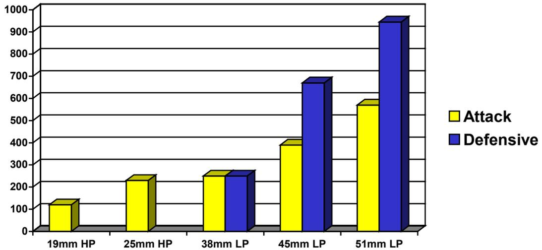
Figure 10 - Flow-comparisons from a range of hose options.
