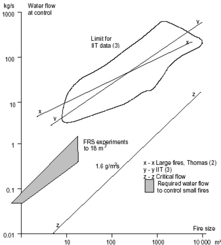
Fig.7 The actual used water flow in relation to the area of the fire is shown. The data are derived from real fires, and taken from reports published in the late 1950's and 1960's. These may not be wholly reliable after forty years - *An Engineering Approach to Firefighting Tactics, Stefan Sardqvist 1996, Report 1014 Lund University Sweden*
