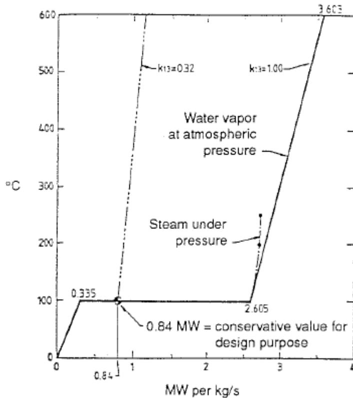
Figure 9 - Cooling power of water applied to a fire at the rate of 1 kg/s (1 litre/s)
