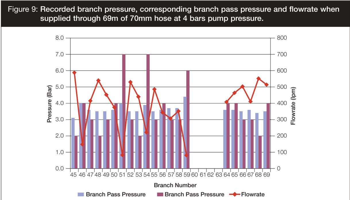
7.13 At 4 bars pressure branches 45, 46, 47, 48, 49, 52, 53, 55, 57, 58, 66, 67, and 68 attained a branch pressure equal or greater than the pass pressure required for the branch (flowrates ranged from 148 to 588 lpm).
