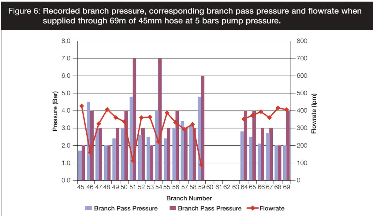
7.8 At 5 bars pressure branches 46, 47, 48, 53, 57, 58 and 68 attained a branch pressure equal or greater than the pass pressure required for the branch (flowrates ranged from 161 to 416 lpm).
