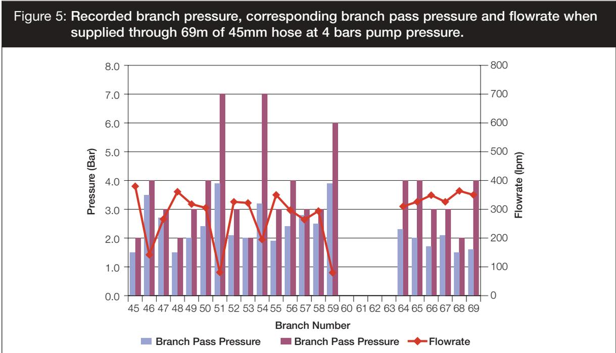
7.7 Of the branches assessed only one branch (branch 53) attained a branch pressure equal or greater than the pass pressure required for the branch (with a corresponding flowrate of 322 lpm).
