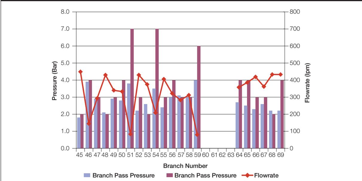
7.10 At 4 bars pressure branches 48, 53, 57, 58 and 68 attained a branch pressure equal or greater than the pass pressure required for the branch (flowrates ranged from 283 to 433 lpm).
