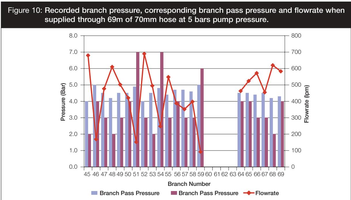
7.14 At 5 bars pressure branches 45, 46, 47, 48, 49, 50, 52, 53, 55, 56, 57, 58, 64, 65, 66, 67, 68 and 69 attained a branch pressure equal or greater than the pass pressure required for the branch (flowrates ranged from 169 to 690 lpm).
