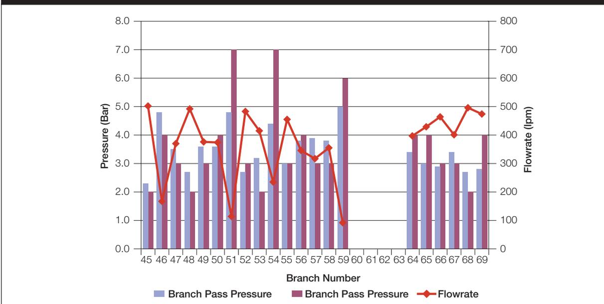
7.11 At 5 bars pressure branches 45, 46, 47, 48, 49, 53, 55, 57, 58, 67 and 68 attained a branch pressure equal or greater than the pass pressure required for the branch (flowrates ranged from 167 to 502 lpm).
