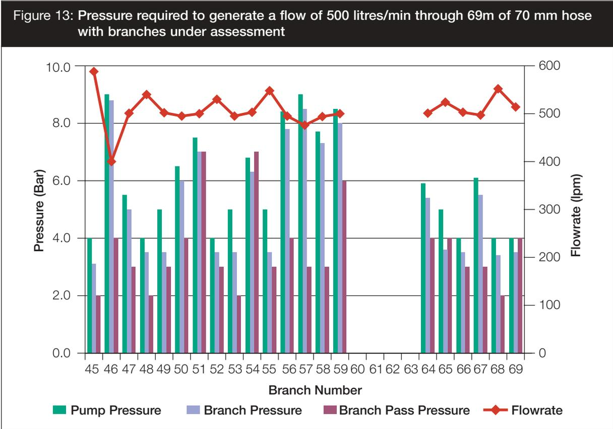
7.18 This shows branches 45, 47, 48, 49, 50, 51, 52, 53, 54, 55, 56, 58, 59, 64, 65, 66, 67, 68, 69 all achieved the required flowrate of 500lpm at pump pressures ranging from 4.0 to 8.5 bar. The remaining branches would be able to achieve a flowrate of 500lpm but these would require in excess of 9 bar pump pressure.
