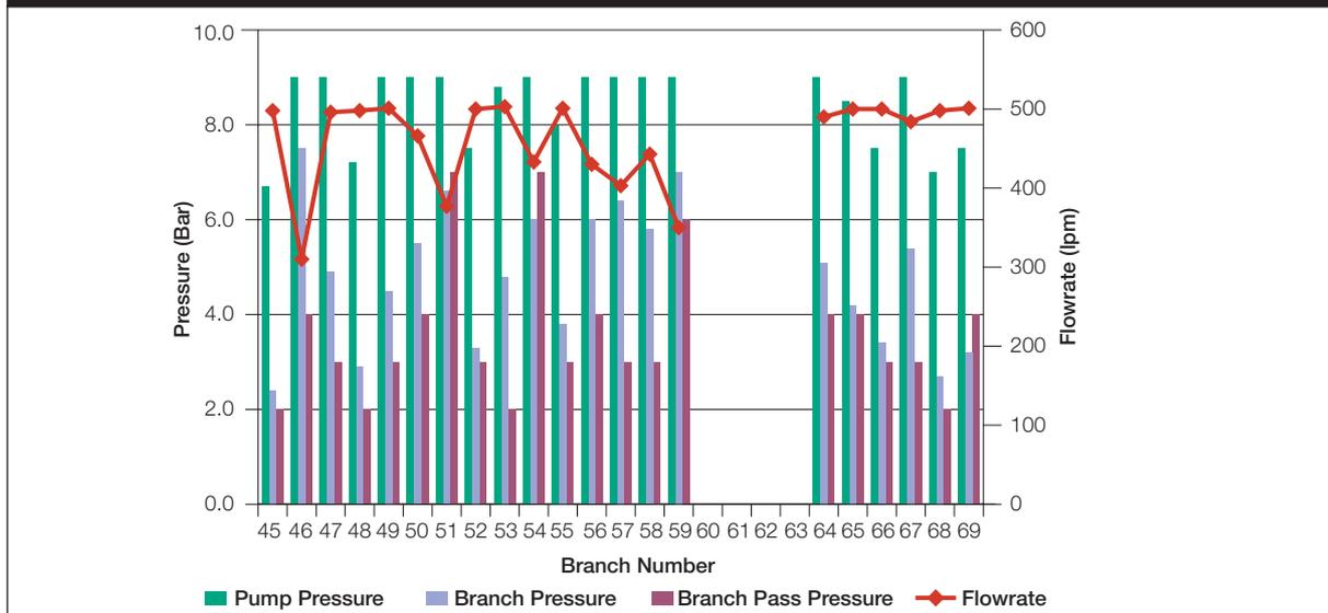
7.16 This shows branches 45, 47, 48, 49, 52, 53, 55, 65, 66, 68, 69 all achieved the required flowrate of 500lpm at pump pressures pressures ranging from 6.7 to 9.0 bar. The remaining branches would be able to achieve a flowrate of 500lpm but these would require in excess of 9 bar pump pressure.
