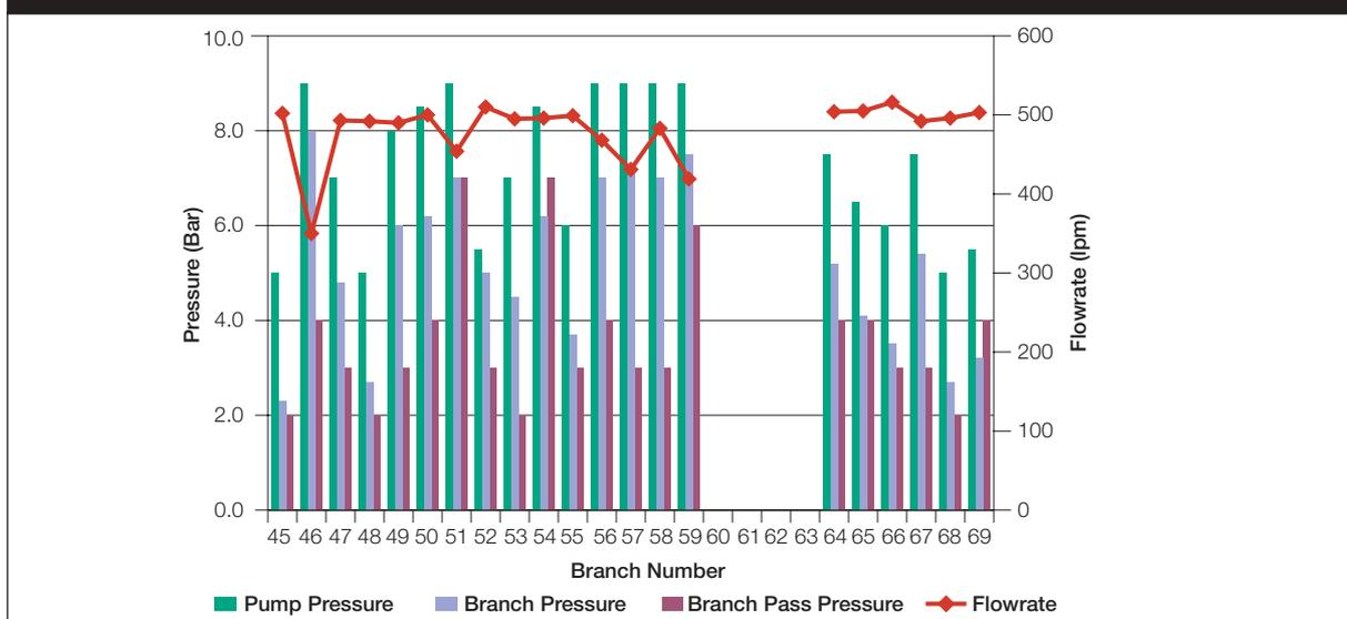
7.17 This shows branches 45, 47, 48, 49, 50, 52, 53, 55, 64, 65, 66, 67, 68, 69 all achieved the required flowrate of 500lpm at pump pressures pressures ranging from 5.0 to 9.0 bar. The remaining branches would be able to achieve a flowrate of 500lpm but these would require in excess of 9 bar pump pressure.
